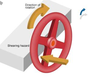
Shearing – a finger put through the spokes of this wheel will be sheared off
