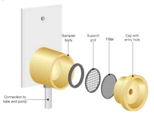
Dust sampler head showing filter in position (Based on original source: MDHS 14/3 General Methods for Sampling and Gravimetric Analysis of Respirable and Inhalable Dust) (Reproduced under the terms of the Open Government Licence)
