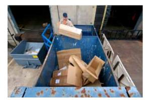
Worker loading a waste compactor. Note the compactor is for cardboard only. Also note the access platform to give safe access to the edge of the skip
