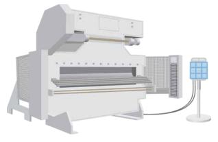
A photoelectric device fitted to a press brake; the device forms a curtain of beams across the front of the machine (Based on original source L22 Safe Use of Work Equipment)
