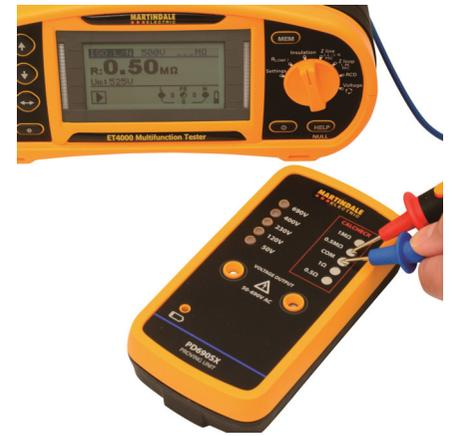
potential calibration issues with test equipment prior to certifying a new wiring installation or carrying out a condition report. This is a procedure recognised by electrical contractor assessment bodies.
