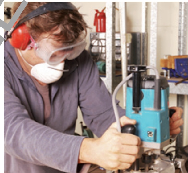
A Worker Wearing a Filtering Face-Piece Respirator to Prevent Inhalation of Wood Dust
