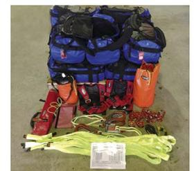
Survitec will provide a range of items including full body harnesses, rescue slings, shock absorbing lanyards, static ropes, karabiners, pulleys and other components to create 35 standard packs of equipment that can be easily carried in a portable holdall. An additional three packs will be supplied with a slightly different configuration. All the equipment conforms to BS EN standards and it is supplied with Kent FRS unique identification numbers laser etched into the products.
