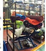
the stillage to a comfortable height to lift off the fabric roll. From a trial with one lift table the cutting area now has four since it proved to be a effective improvement to the working system and gave improved operator safety.
